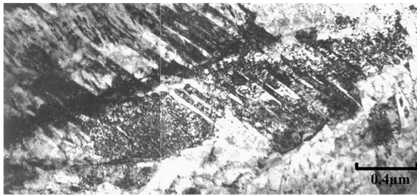
Fig. 9 Transmission electron micrograph showing the microstructure of irregular-shaped tempered twinned plate martensite formed in the specimen after the third stage ( 3 \times 1 h) tempering at 650^\circ\text{C} and cooling to room temperature
