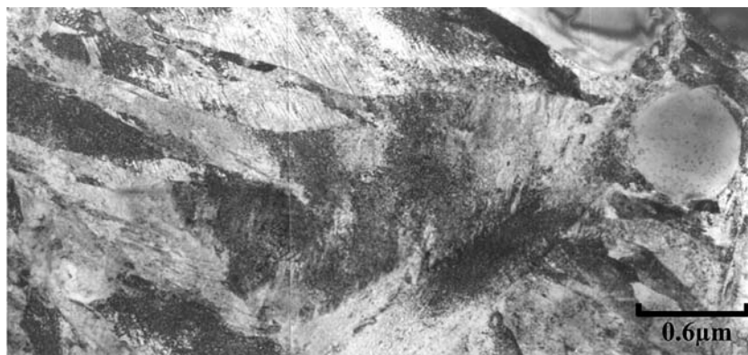
Fig. 5 Transmission electron micrograph showing the microstructure of the degenerated structures in twinned plated martensite and adjacent austenite
